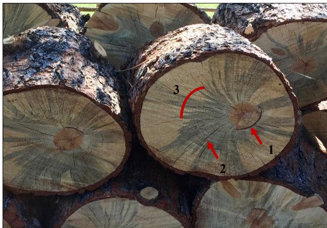
Examples of damage following a storm: 1) ring shake, 2) cracks, 3) beetle-vectored stain
